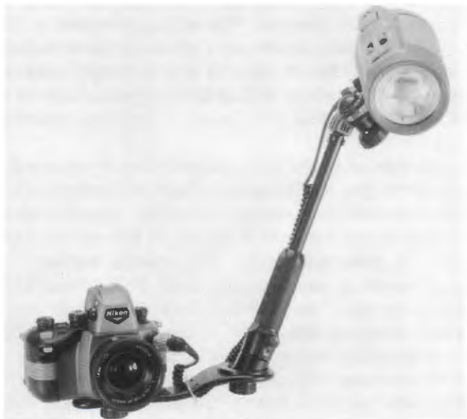
271. A flash bracket helps position the flash properly off-camera so that particles suspended in the water will not reflect light from the flash directly back to the camera. This helps prevent an annoying problem in underwater photography known as backscatter.
