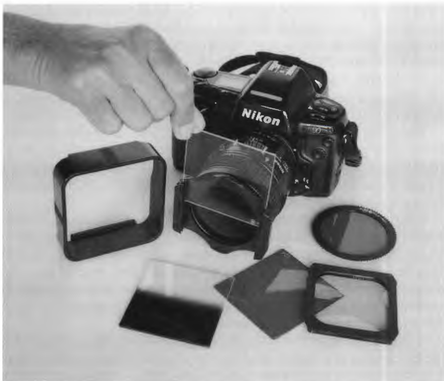
147. Filter systems by Cokin and other filter manufacturers offer an extensive variety of filters that slip into a filter holder that's screwed onto the camera lens. In order to use the filters on all your lenses, make sure they'll cover the lens that has the largest diameter.
