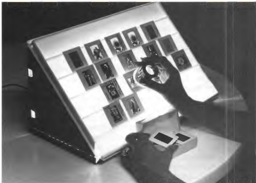
314. A convenient way to preview and edit your color slides before projecting them is to study the slides through a hand-held magnifier, known as a loupe. Then arrange them in order on an illuminated slide sorter, also called a light box.
