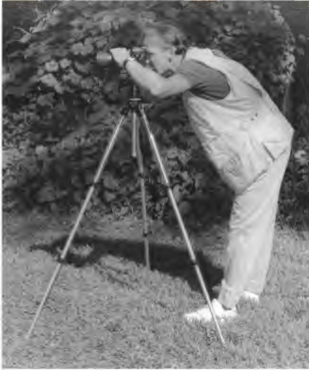
167. Position a tripod so that one leg is pointed in the direction of the camera lens. That way you'll have room to stand between the two legs at the rear and avoid tripping over the tripod.
