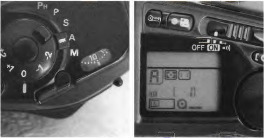
50. Single lens reflex (SLR) cameras featuring multimode exposure have an exposure mode selector or control dial for choosing programmed (P), shutter-priority (S or Tv), aperture-priority (A or Av), or manual (M) exposure. These two cameras have been set to aperture priority (A).
