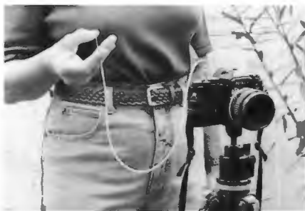
165. When making time exposures, you can use a cable release to trigger cameras that have a mechanically controlled shutter, thus avoiding blurred images that can result from inadvertent camera movement.
