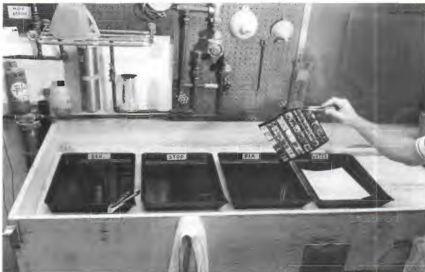
292. When processing a black-and-white proof sheet, or an enlargement, print tongs are used to transfer the photo paper from one solution to another: developer to stop bath to fixer to wash water.
