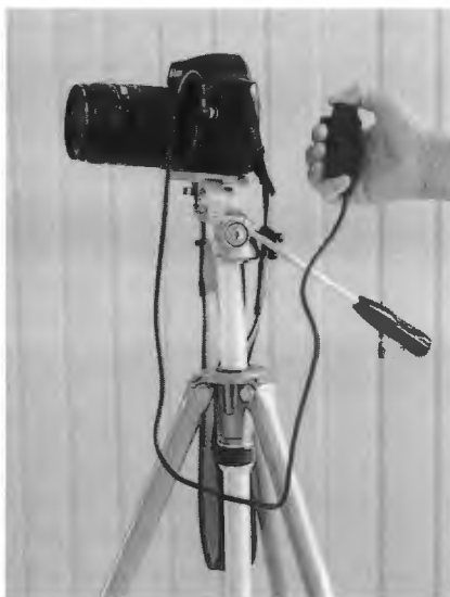
166. For cameras with an electronically controlled shutter, a remote cord can be used to trigger the shutter release without touching the camera.
