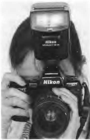
106. Of the several types of flash equipment, shoe-mount flash is most often used with 35mm single lens reflex (SLR) cameras.
