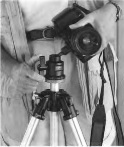
168. A ball head on a tripod makes it easy to turn a camera from a horizontal position to a vertical position or to any other angle.
