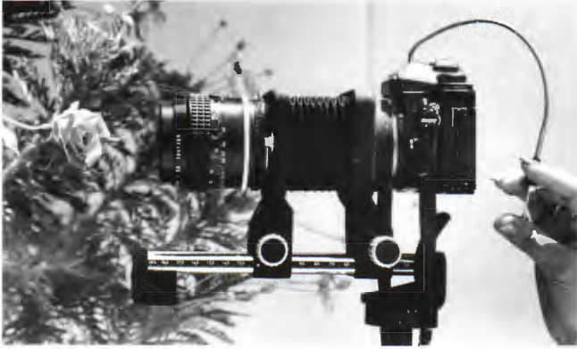
99. For versatility in making close-up photographs, an adjustable extension bellows can be mounted between the camera body and the lens. Here it is being used to show the interior of a flower (see Illustration 98). Because of the great magnification, the bellows is mounted on a tripod for support; a cable release is used to prevent the camera from being moved inadvertently during the exposure.
