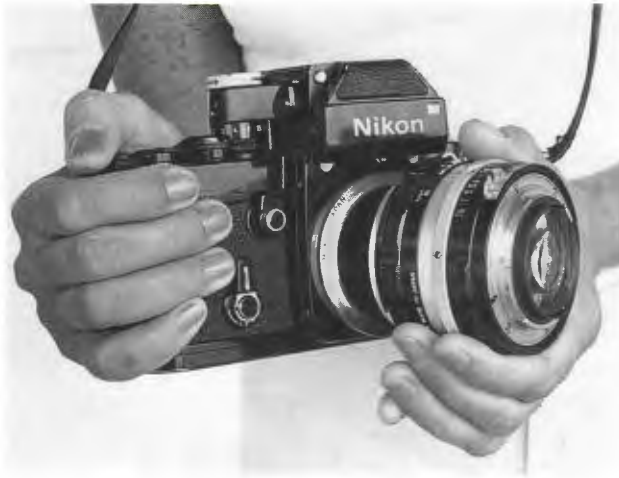
251. A simple way to make extreme close-up photographs with a single lens reflex (SLR) camera is to turn a normal or wide-angle lens end for end and remount it to the camera with a lens reversing ring (see text).
