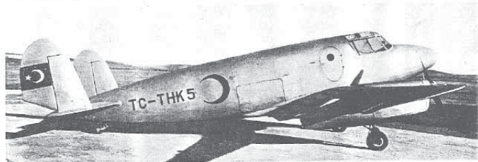
The T.H.K. 5A Light Ambulance (two 135 h.p. D.H. Gipsy Major engines).
