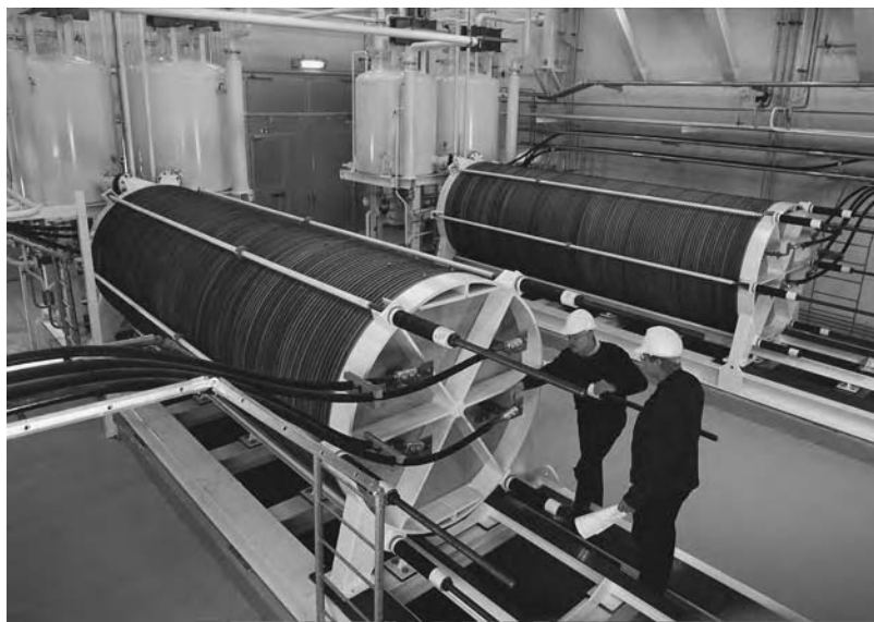
FIGURE 2.1 (a) Schematic of water (alkaline) electrolysis. (b) Two large ( 200 \text{ Nm}^3/\text{h} ) atmospheric, alkaline, multicell electrolysis stacks generating hydrogen at the Norsk Hydro Company.
