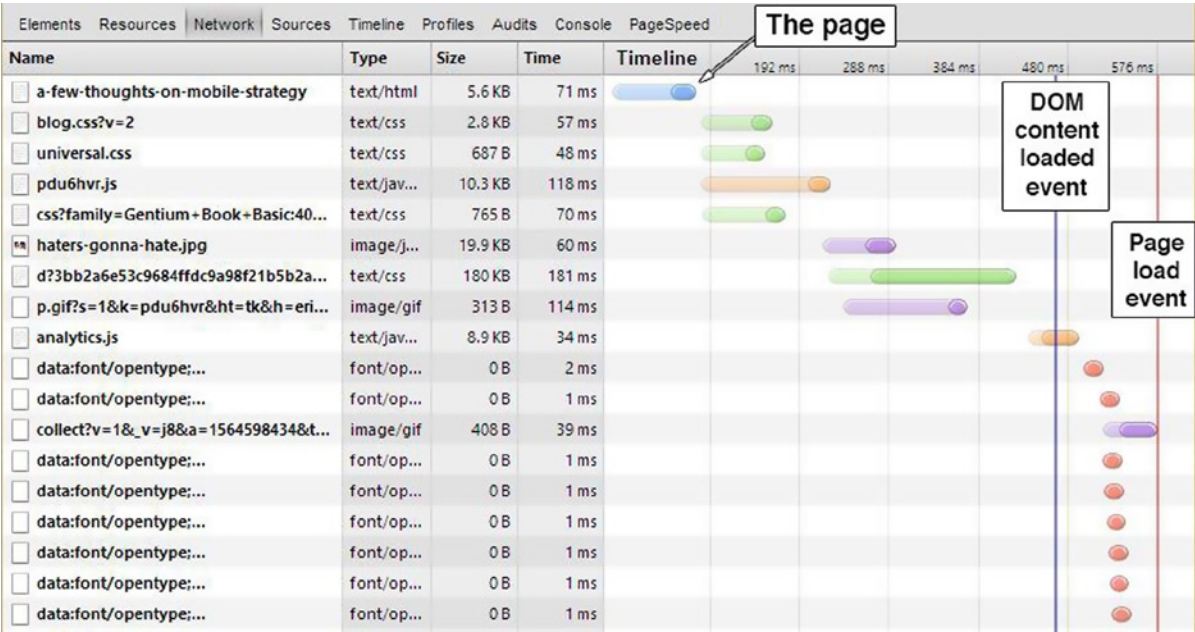
Figure 8-1. The Network tab of the Chrome developer tools. This is a screenshot taken while browsing one of my unoptimized websites
