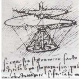
Leonardo's flying machine. He made detailed observations of bats and birds to see how they flew, but his own machine lacked the power to take off. (Leonardo wrote all his notes from right to left with the letters reversed.)
