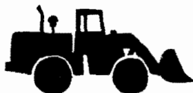
Articulated Loader (pivots in center)
