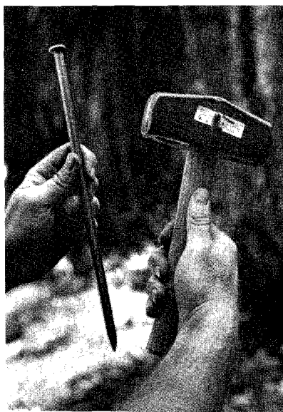
A bridge timber spike and single jack hammer for use with very large trees. Smaller spikes are fine for general use and can be driven in with a heavy standard hammer.
