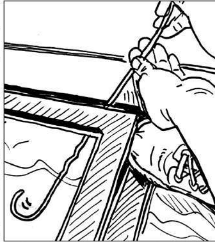
Use shoe toe as wedge to keep gap open. Insert hanger to hit unlock button, pull door handle, or retrieve keys.
